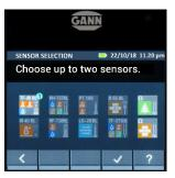
Sensors that are connected to the measuring device are visually high-lighted and can be selected.
