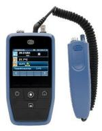
The active electrode TF-IR BL must be connected to the measuring instrument via the 3.5 mm jack receptacle. Ensure that the octagonal plug is firmly seated. The measuring instrument now automatically recognises the connected accessories.
