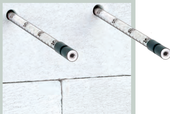
DETAIL Both electrode pairs are equipped with one-centimetre division scale
