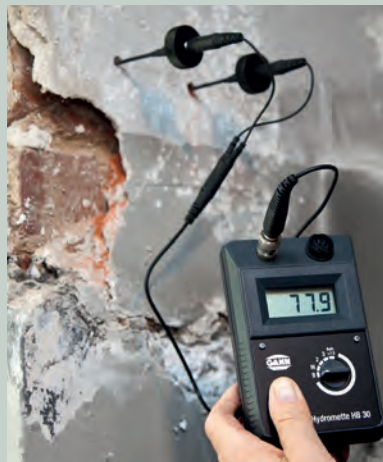
APPLICATION HB 30 together with an M 25-100 brush electrode pair
