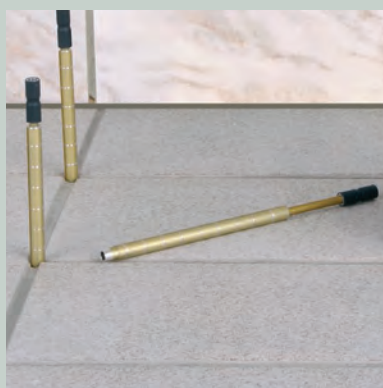
DETAIL Both electrode pairs are equipped with one-centimetre division scale
