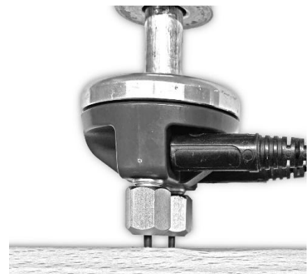
Figure 14-2: Use of Teflon-insulated pins
