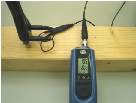
Figure 4-1 Measurement across the grain with M 20
