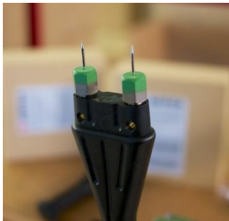
Figure 4-3 Wood fibre insulating material electrode on M 20 electrode
