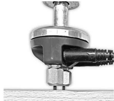
Figure 13-2: Use of Teflon-insulated pins
