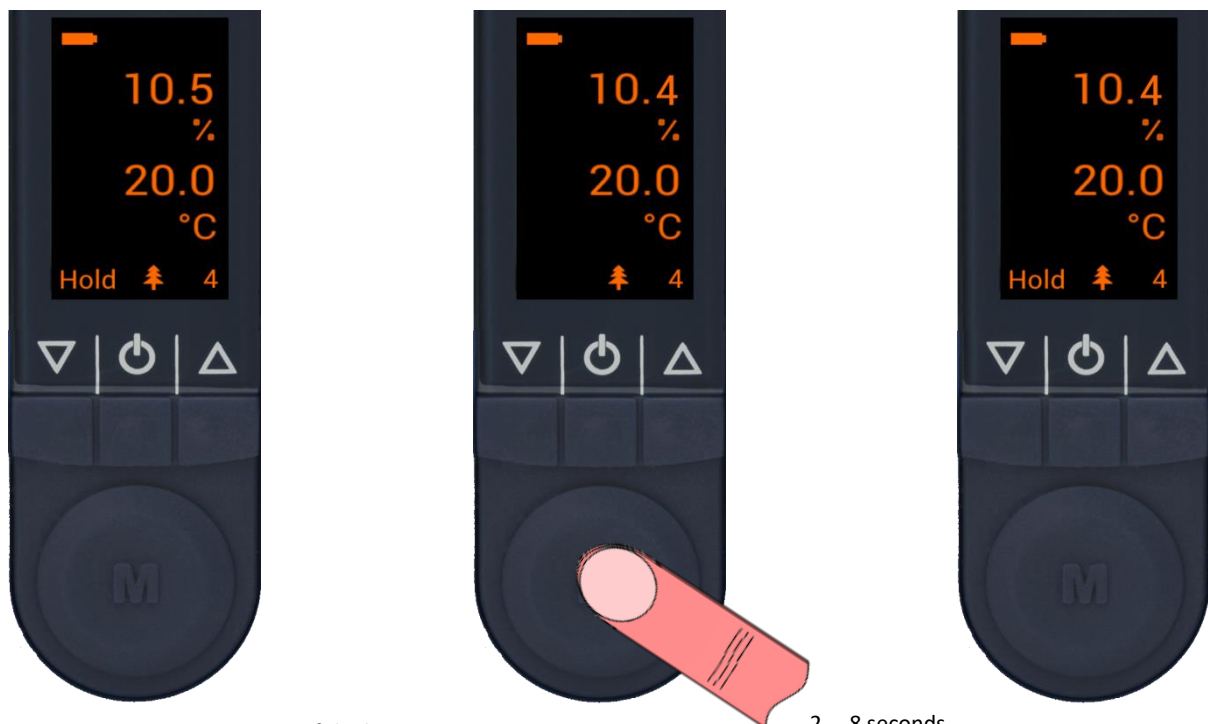
Figure 8 2: Measuring process of the basic measurement
