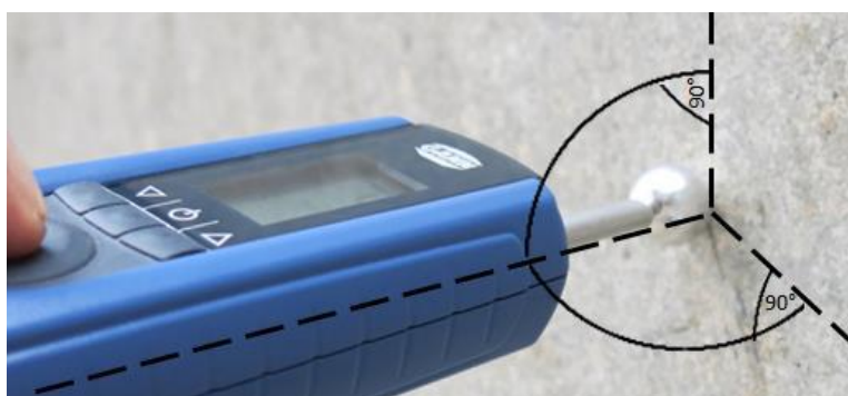
Figure 13-3: Measuring as vertically as possible to the measurement area
