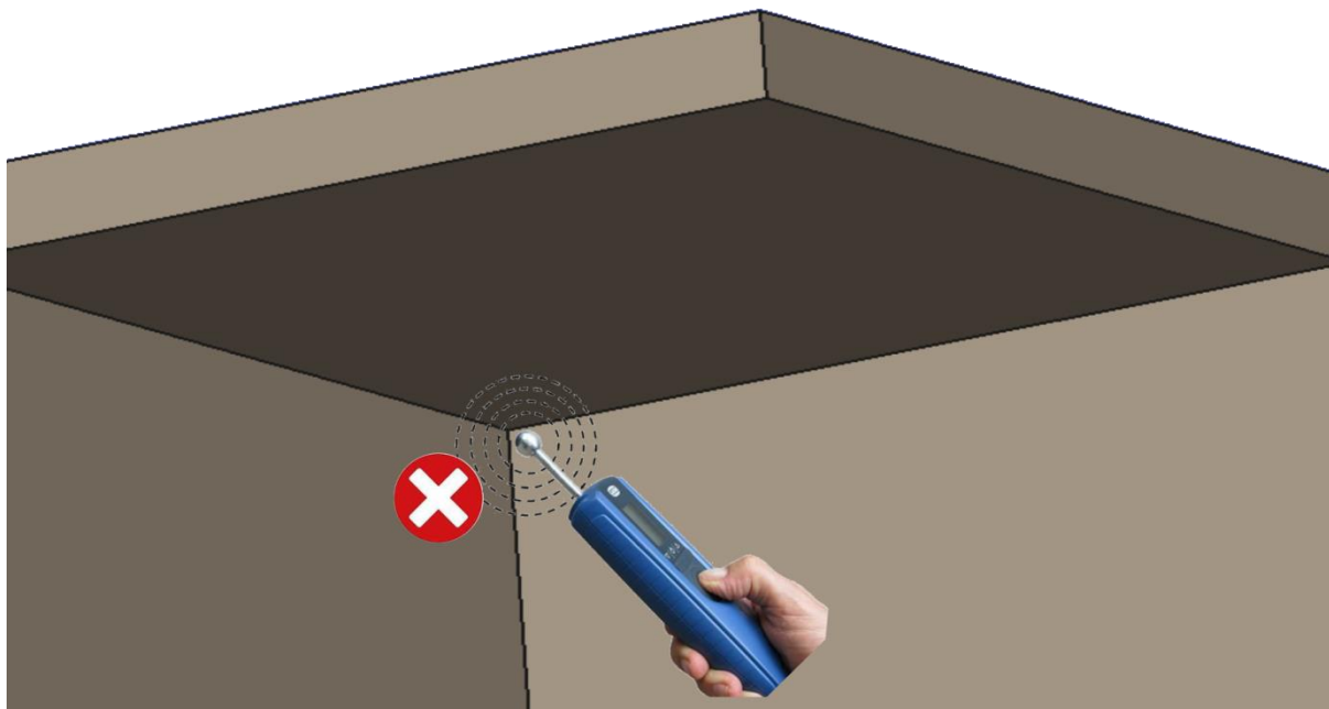
Figure 13-6: Incorrect use in corner/angle area
