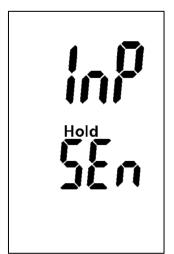
If the TF-stick is not (correctly) inserted, the display "InP SEn" is shown when the measuring button is pressed and held down for a *long time* (>2 seconds)!
