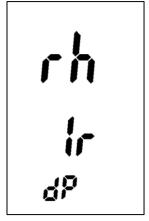
Figure 6-1: Measuring mode selection "Dew point IR"
