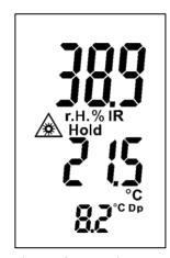
Figure 5-9: Measuring menu "Dew point IR"
