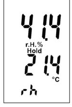
Figure 5-13: Measuring menu "relative humidity, rh"
