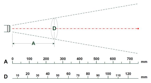
Figure 9-1: Measurement spot size depending on distance
