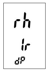
The device is delivered with the measuring mode "Dew point IR" (rh / lr / dp) as factory setting.
