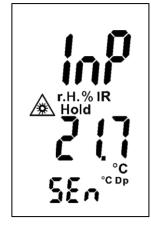
Figure 6-2: Measuring menu "Dew point IR" without TF-Stick
