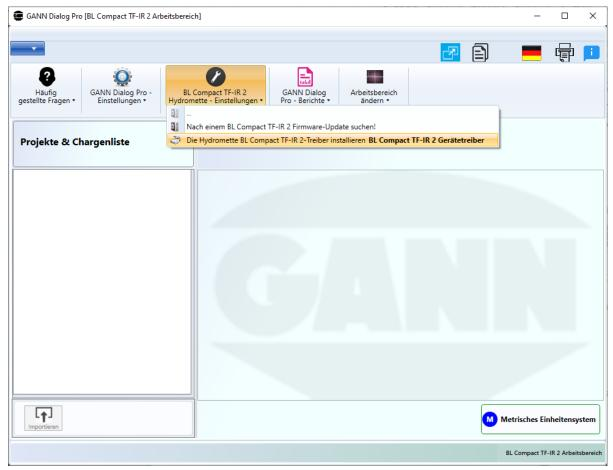
Figure 7-2: Download device drivers of the Hydromette BL TF-IR 2  $\,$
