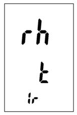
Figure 5-10: Measuring mode selection "Surface temperature IR"
