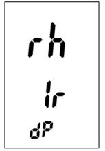
Figure 5-8: Measuring mode selection "Dew point IR"
