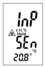
Figure 6-4: Measuring menu "Surface temperature IR" without TF-Stick
