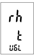
Figure 5-18: Measuring mode selection "Equilibrium wood moisture content, EMC"
