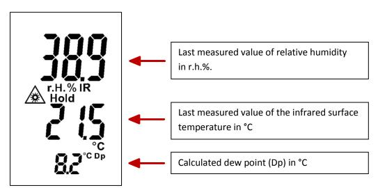
Figure 5-4: Standard Measuring Menu
