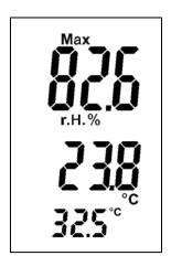
deletion of the value. The device returns to the measuring mode by *briefly* (< 1 second) pressing the "**M**" button again.
