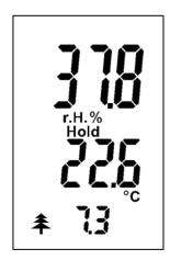
Figure 5-19: Measuring menu "Equilibrium wood moisture content, EMC"
