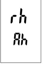
Figure 5-20: Measuring mode selection "absolute humidity, Ah"
