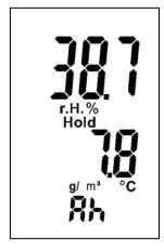
Figure 5-21: Measuring menu "absolute humidity, Ah"
