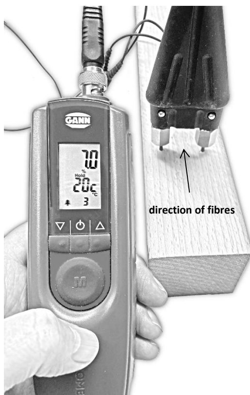
Figure 9-1: Wood moisture measurement – perpendicular to direction of fibres
