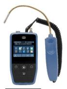
The active electrode RH-T 37 BL flex must be connected to the measuring instrument via the 3.5 mm jack receptacle. Ensure that the octagonal plug is firmly seated. The measuring instrument now automatically recognises the connected accessories.
