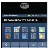
To activate the RHT measurement mode, the "RH-T 37 BL flex" symbol must now be selected. The selection is confirmed by pressing the "Confirm" button.
