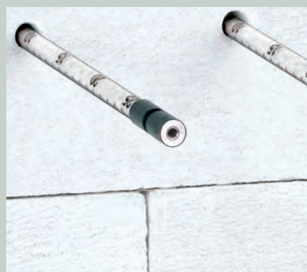
DETAIL Both electrode pairs are equipped with one-centimetre division scale
