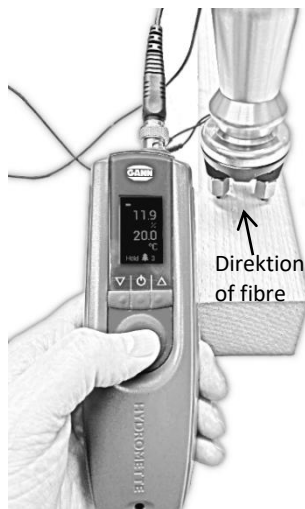
Figure 3-1: Wood moisture measurement – perpendicular to direction of fibres
