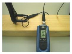
Figure 4-1 Measuring across the fibre direction with M 20
