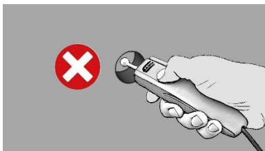
Figure 5-3: Incorrect use – measurement in drill hole
