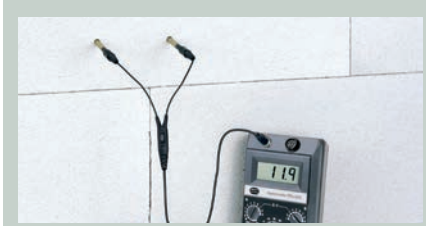
APPLICATION Measuring structural moisture using the RTU 600 unit and an M 21-100 deep measuring electrode pair
