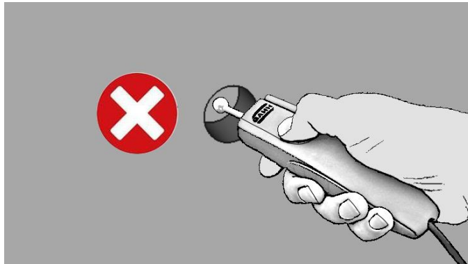
Figure 13-5: Incorrect use – measurement in drill hole
