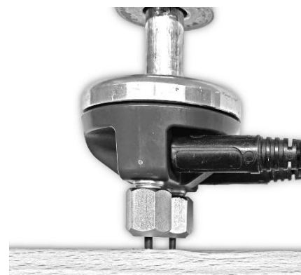
Figure 13-1: Use of Teflon-insulated pins
