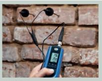
APPLICATION Measurement of structural moisture in bricks using an M 25-100 brush electrode pair
