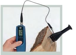
APPLICATION Moisture measurement perpendicular to the wood fibre direction using an M 20 electrode
