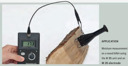
on a wood billet using the H 35 unit and an
