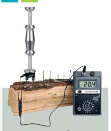
APPLICATION Hydromette<sup>®</sup> HT 85 T unit together with an M 18 ram-in electrode
