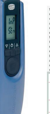
The BL UNI 11 unit is an electronic multi-purpose meter for three measured values. It can be used with a number of blue product series electrodes and TF sticks. Electrodes for measuring structural moisture, air humidity, and temperature may be connected.
