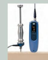
Resistance-based measurement in hardwood using an M 18 ram-in electrode
