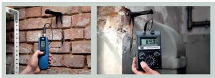
APPLICATION A hammer may facilitate the drive-in of the M 20 electrode
