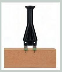
M 20 drive-in electrode with special insulated electrode nuts that reduce the impact of surface moisture
