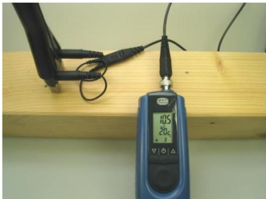
**Figure 4-1 Measuring across the fibre direction with M 20**
